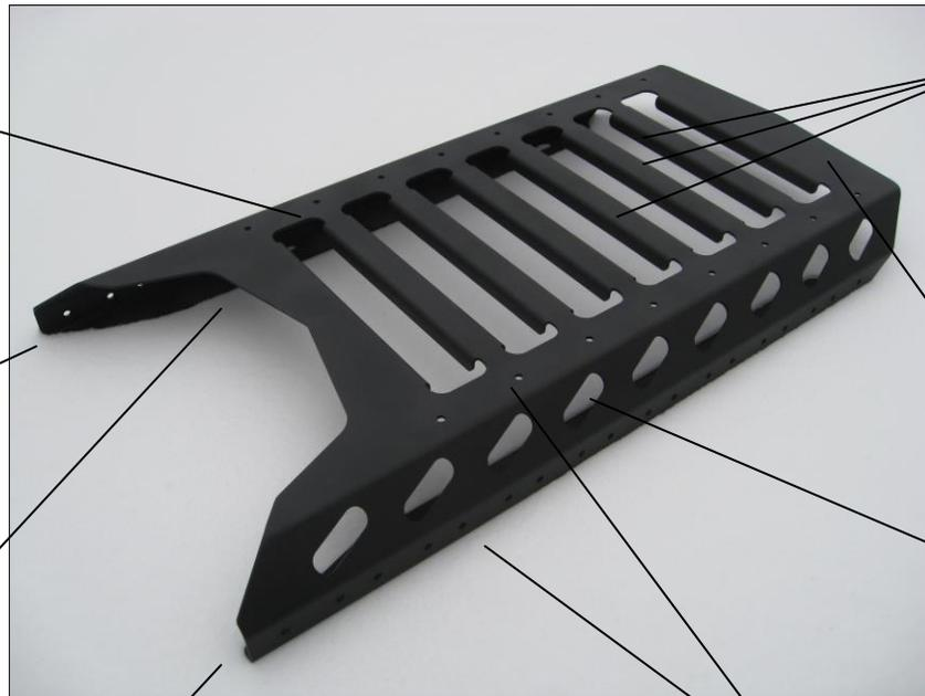
Cargo deck surface is elevated above the tunnel and heat exchanger, eliminating exposure to heat, moisture, and abrasion
