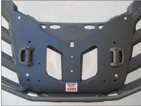
ATV-1 LINQ™ ADAPTER BRACKET INSTALLED ONTO STOCK CAN-AM® OUTLANDER™ RACK
