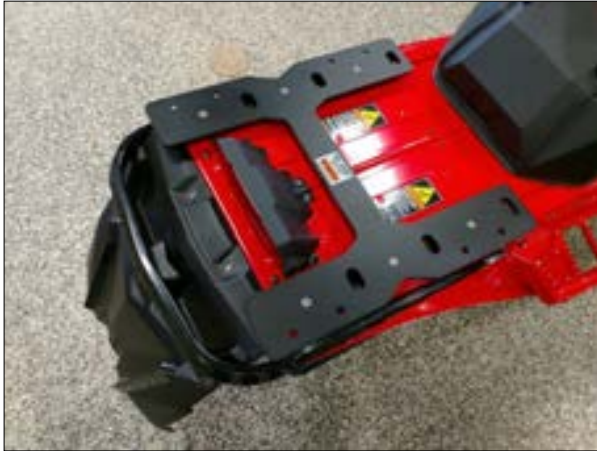
LMP-129-XC DUAL-POSITION LINQ™ ADAPTER BRACKET INSTALLED ONTO THE 2019 POLARIS® INDY XC™
