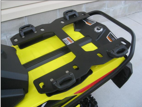
LMP-129 DUAL-POSITION LINQ™ ADAPTER BRACKET INSTALLED ONTO THE SKI-DOO® REV™ G4 MXZ™
