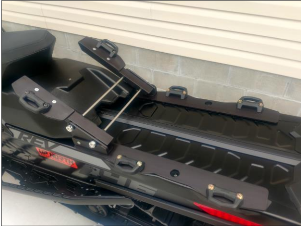
X3 TRIPLE LINQ™ ADAPTER SYSTEM INSTALLED ONTO SKI-DOO® REV™ G4 SUMMIT™ SP 146
