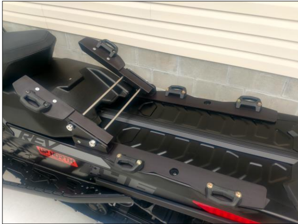
X3 MOUNTAIN TRIPLE-POSITION LINQ™ ADAPTER SYSTEM INSTALLED ON SKI-DOO® REV™ G4 SUMMIT™ SP 146
