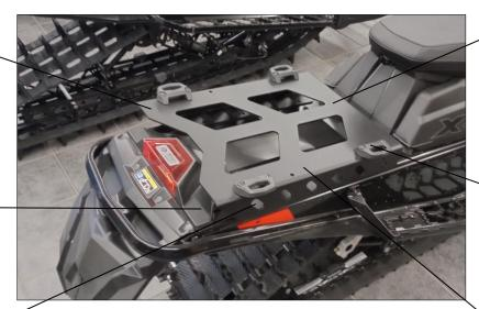
UP NORTH TECHNOLOGIES, INC. The top surface of the **CR137 COMBO RACK** is above the taillight,
